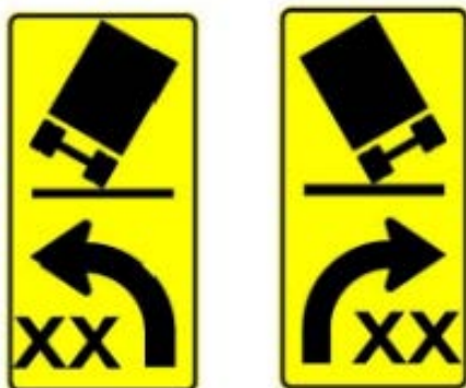
Figure 6.55: Truck tilting warning signs with advisory speed.
