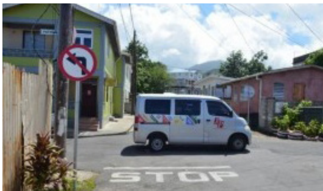
Figure 6.8: No left turn sign with stop marking at unsignalized intersection in Dominica.
