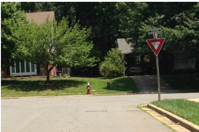
Figure 6.3: Yield signs being used as intersection control.
