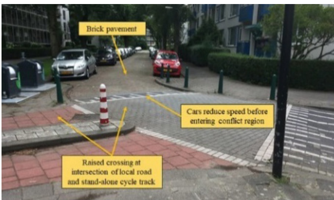
Figure 6.50: Raised intersection with different pavement pattern.
