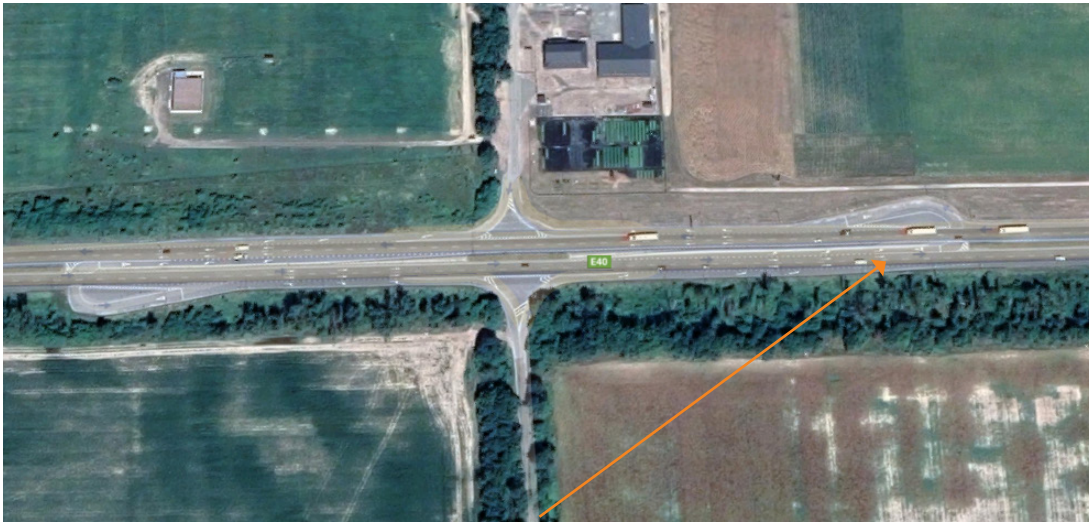
Figure 6.74: RIRO junction with too close offset right turn in Ukraine.
