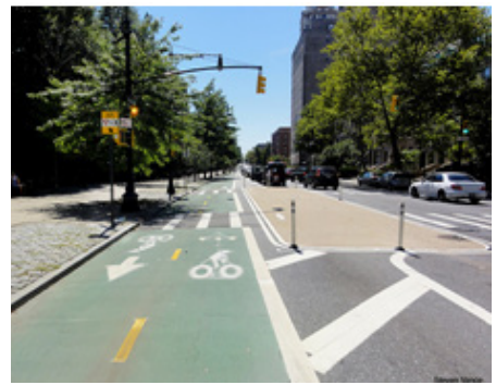
Figure 6.66: Pedestrian refuge and cyclist way finding.
