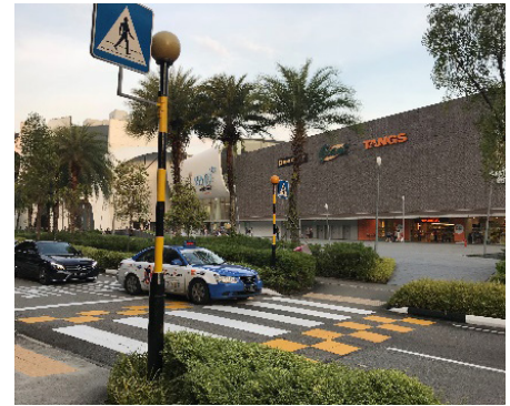
Figure 4.22: Well defined crossing with signing—Singapore.
