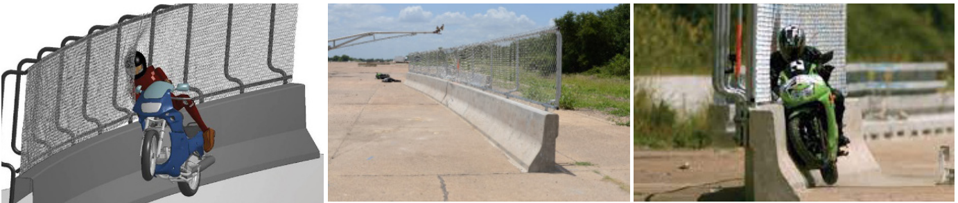
Figure 4.56 Modified U-shaped posts and attached to a curved concrete barrier
