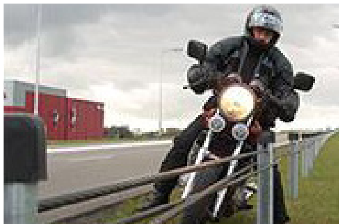
Figure 4.52: Motorcyclist impact with wire rope barrier.
