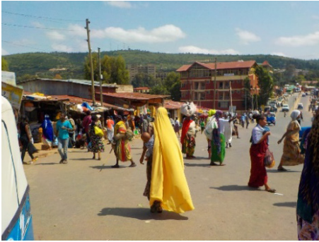
Figure 3.22: No footpath or crossing facility for pedestrians.
