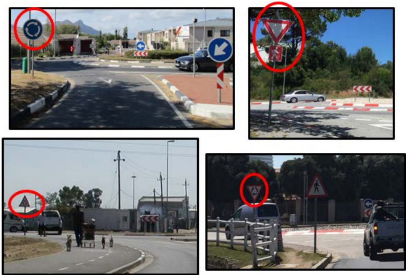
Figure 6.42: Good quality roundabout sign but variation of sign in the same country confusing drivers in South Africa.
