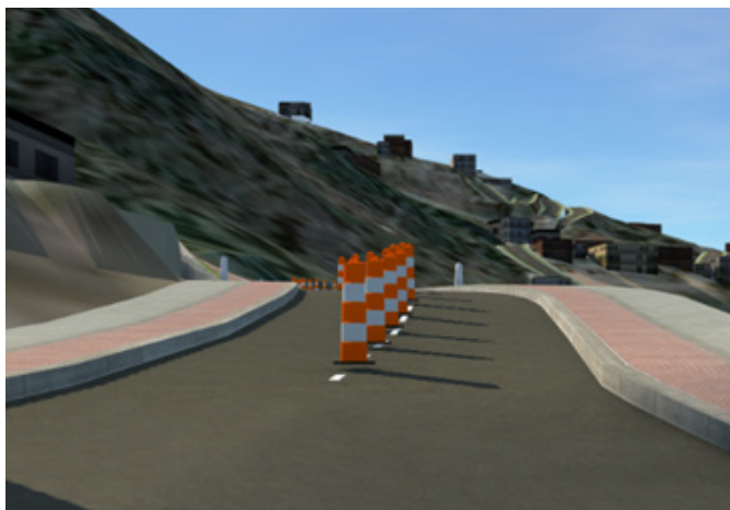
Figure 5.51: Illustration on provision of flexible posts at curves with limited sight distance.
