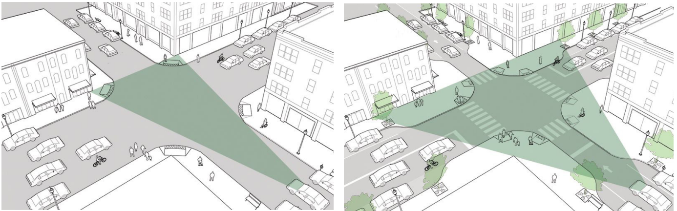
Figure 3.18: Examples of driver's sight triangles at intersections
