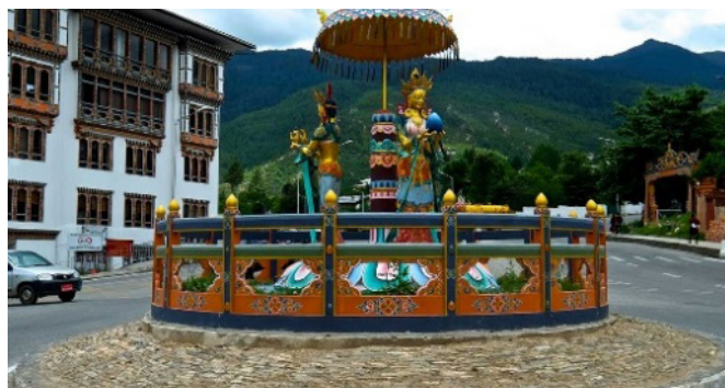
Figure 6.33: Decorated roundabout obscuring driver's sight in Bhutan
