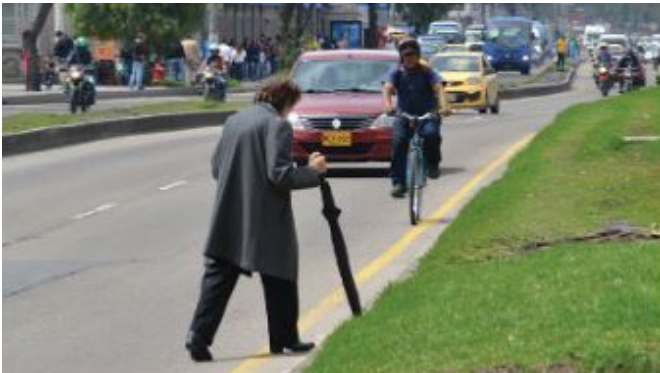
Figure 5.2: Use of wide lanes in an urban area at the expense of vulnerable users (pedestrians and cyclists).
