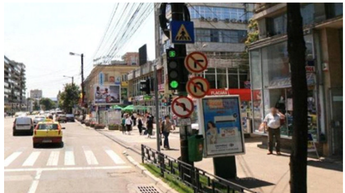
Figure 5.162: Overuse of signs is distracting.
