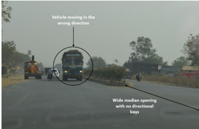
Figure 5.112: Unsafe median opening leading to contraflow.
