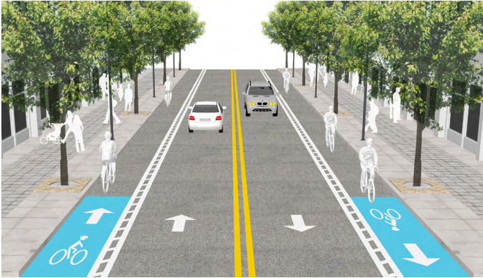
Figure 19. Uni-directional marked cycle lane.
