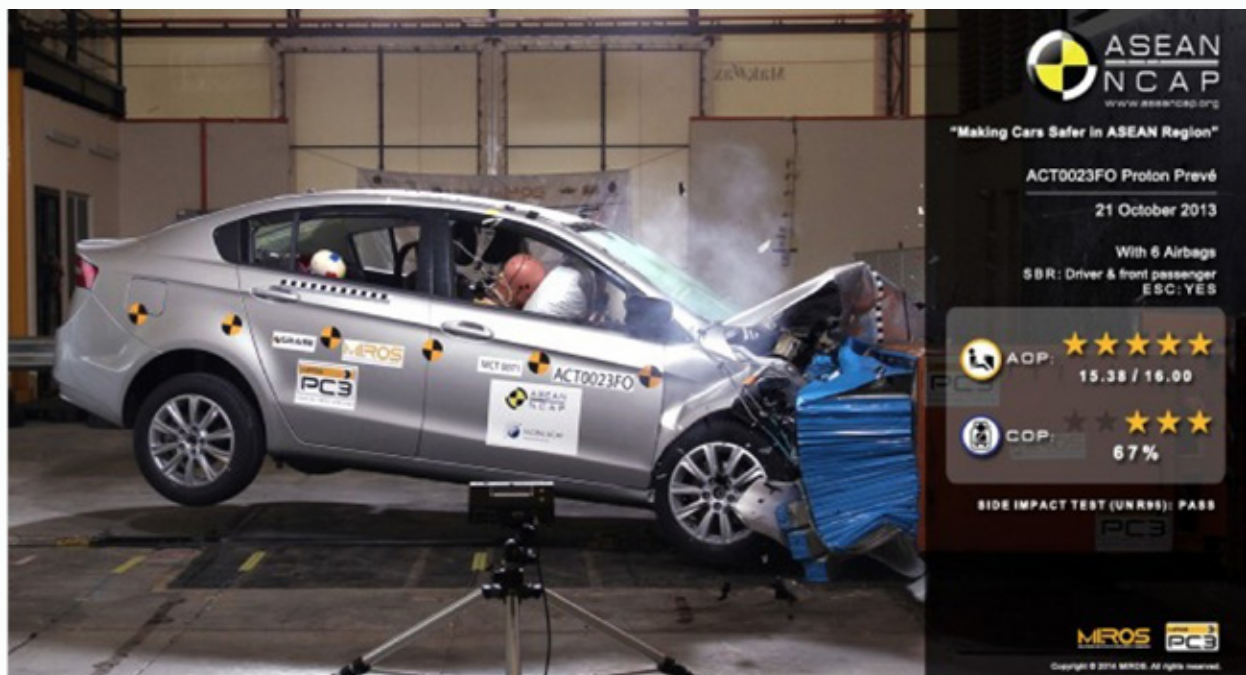
Figure B2.4.1 ASEAN NCAP Collision Test Conducted in the MIROS Testing Laboratory
