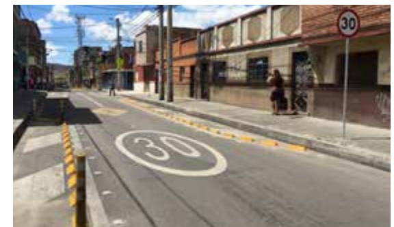
Figure 10.12 | Medium-Term Materials Installed in Tunjuelito to Form a Choker after Success of the Temporary Pilot Project
