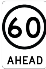
Figure 1: Example of an advanced warning sign (Speed Limit Ahead), sign no. G9-79
