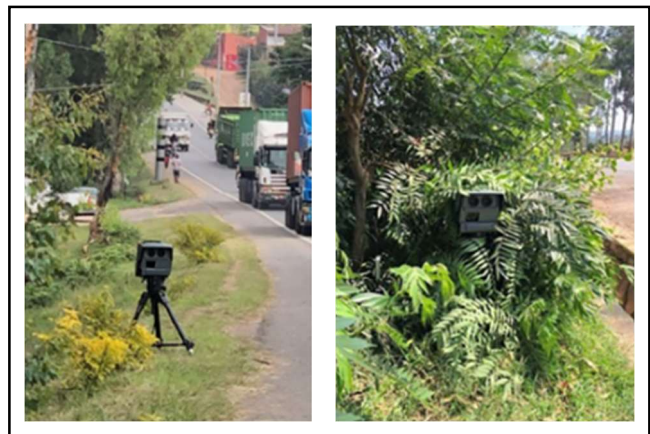
A visible (left) and hidden (right) speed camera used in the study.
