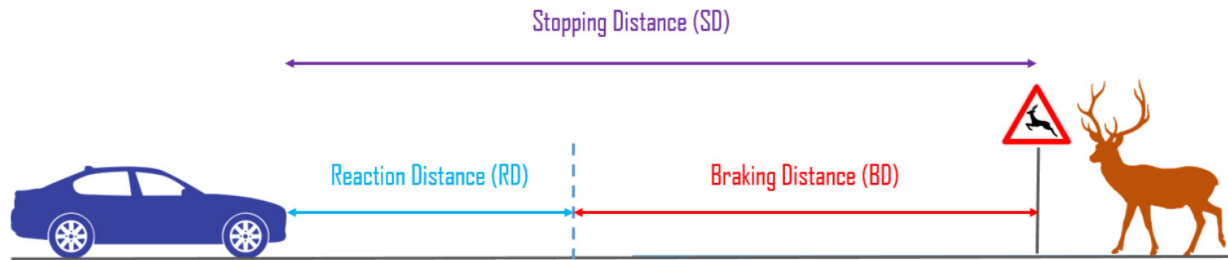
Figure 2.1. At higher speeds drivers need longer distance to react, process and brake to stop.
